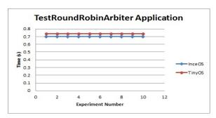
The TestRoundRobinArbiter application results are displayed in Figure 12, again showing an InceOS performance gain when compared to TinyOS. Here the 36 ms gain is because the Insense channel abstraction is used in InceOS to arbitrate access to the shared resource, whereas additional functionality is required for such arbitration using TinyOS. This particular application is well-suited to the Insense blocking channel interaction which naturally handles arbitration.
