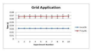
The results for the grid application are shown in Figure 11. Here the time for a complete iteration of the application is taken: request a slave, give it work and collect the reply. We see that InceOS performs
