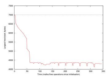
Fig. 5. External fragmentation: largest free block in the interpreted *Ra-dioSenseToLeds* application.
