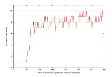
Fig. 4. External fragmentation: number of free blocks in the interpreted *RadioSenseToLeds* application.
