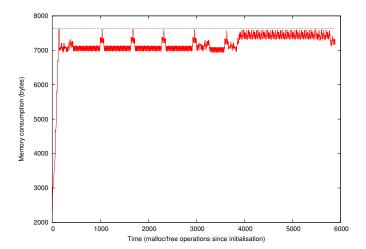
Fig. 6. Dynamic memory usage of the DataLogger application.
