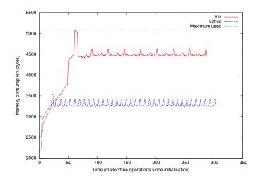
Fig. 3. Dynamic memory usage of the RadioSenseToLeds application.
