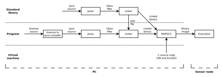
Fig. 2. Compiling and executing an Insense program. The 'split VM' architecture is shown by the separation between PC and sensor node.
