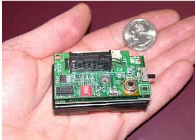
Figure 1.1: Mote beside an American 25c coin. Intel Research, Berkeley [16]
